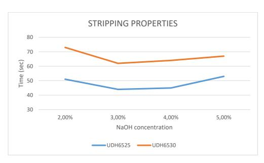
Data in the graph are obtained with laboratory dipping test; Exposure at SST13/41; Flake size: Sheet
