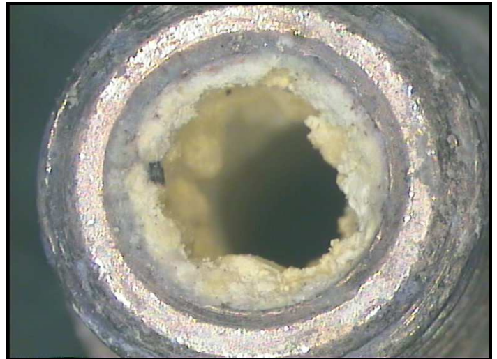
Nozzle before cleaning
